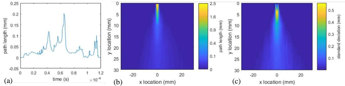
**Figure 3:** Data available from focused beam measurements with  $Re_l = 1,000$ ,  $Re_g = 16,700$ , and  $SR = 0$  (a) short clip of path length as a function of time, taken from  $x=0$ ,  $y=4$  (b) average path length (c) path length standard deviation.
