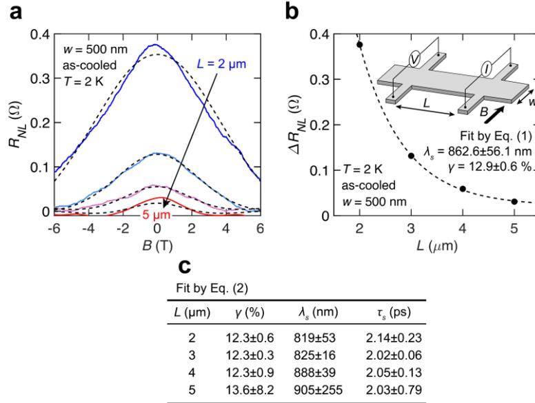
**Figure 2. a**, Non-local resistance,  $R_{NL}$ , as a function of the magnetic field,  $B$ , for probe spacings between  $2 \mu\text{m}$  and  $5 \mu\text{m}$  at  $2 \text{ K}$ . The fit of the data to Eqs. (1-2) is shown as dashed lines. **b**, The non-local resistance amplitude,  $\Delta R_{NL}$ , as a function of probe spacing,  $L$ . **c**, Table of extracted fitting parameters from the fits in **a**.
