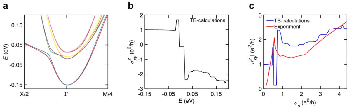
**Figure 4.** *a*, Calculated energy dispersion of the spin-split sub-bands along high symmetry crystal directions. *b*, Calculated spin Hall conductance,  $\sigma_{xy}^z$ , as a function of the energy,  $E$ . *c*, absolute value of  $\sigma_{xy}^z$  calculated and obtained experimentally from  $\gamma$  in Fig. 3c, as a function of the sheet conductance,  $\sigma_s$ . The experimentally observed maxima of  $\gamma$  is reasonably well captured by the calculations.
