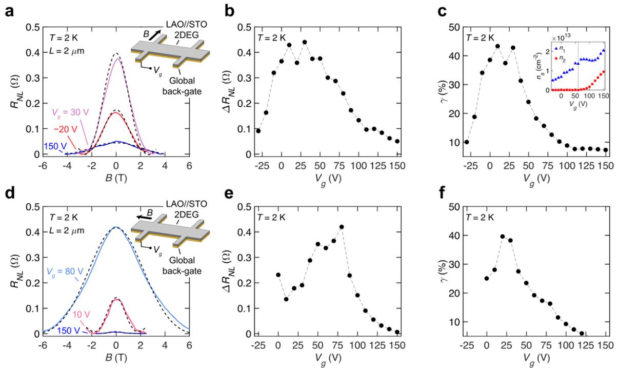
**Figure 3. a**, Non-local resistance,  $R_{NL}$ , as a function of the magnetic field applied along  $x$ ,  $B$ , for three representative gate voltages at 2 K, for a probe spacing of  $2 \mu\text{m}$ . **b**, Non-local spin
