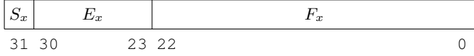
Fig. 8. The IEEE-754 binary32 (a.k.a. single precision) representation of a floating-point number x . The floating-point exponent e_x of x is E_x - 127 , the significand m_x of x is 1 + 2^{-23} \cdot F_x , so that x = (-1)^S \times 2^{E_x-127} \times (1 + 2^{-23} \cdot F_x) .
