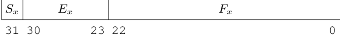
Fig. 8. The IEEE-754 binary32 (a.k.a. single precision) representation of a floating-point number x . The floating-point exponent e_x of x is E_x - 127 , the significand m_x of x is 1 + 2^{-23} \cdot F_x , so that x = (-1)^S \times 2^{E_x - 127} \times (1 + 2^{-23} \cdot F_x) .
