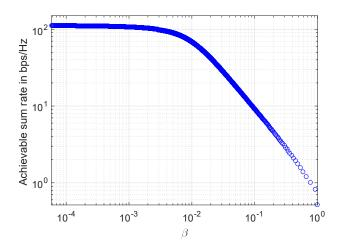
Fig. 2: Case2: Achievable sum rate  $C_D$  averaged over 10,000 simulations for different values of  $\beta$ , defined in (12). Parameters:  $N = 100, D = 99, (p_1 + \dots + p_D)/D = 5, \sigma^2 = 1$ .
