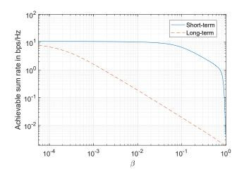
Fig. 4: Case2: Achievable sum rate  $C_D$  for different values of  $\beta$ , defined in (12). Parameters:  $N = 10, D = 9, (p_1 + \cdots + p_D)/D = 5, \sigma^2 = 1.$
