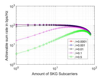
Fig. 1: Case1: Achievable sum rate  $C_D$  averaged over 10,000 simulations for different values of  $\beta$ , defined in (12), number of subcarriers used for data transmission and for SKG. Parameters:  $(p_1 + \cdots + p_D)/D = 5, \sigma^2 = 1, N = 100$ .
