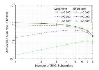
Fig. 3: Case1: Achievable sum rate  $C_D$  for different values of  $\beta$ , defined in (12), number of subcarriers used for data transmission and for SKG. Parameters:  $(p_1 + \cdots + p_D)/D =$  $5, \sigma^2 = 1, N = 10.$
