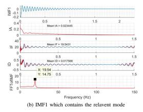
Fig. 5: HHT applied to identify and track coupling mode
