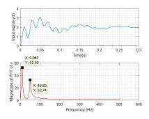
Fig. 1: Input signal and its FFT
