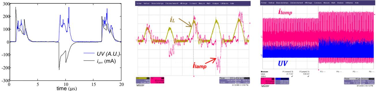
Fig. 6 (a) shapes of the measured instantaneous UV power (blue) compared to the computed  $i_{gas}$  current (black) - (b) instantaneous control of the  $i_{lamp}$  current - (c) UV production controlled by the power supply.
