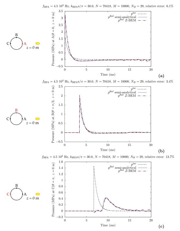
**Figure 8:** Scattering by a large cylinder (a = 5 m, L = 50 m, see Fig. 5): comparison between the Z-BEM and semi-analytical solutions for the total field  $p^{\text{Ref}}$  on the z = 0 plane, at the standoff (a), orthogonal (b) and shadow (c) points. The incident field at those points is also shown.
