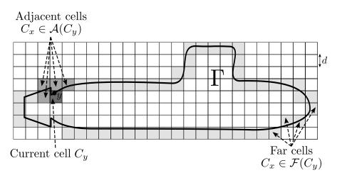
Figure 18: Two-dimensional grid embedding the boundary  $\Gamma$ . Definition of adjacent and far cells.
