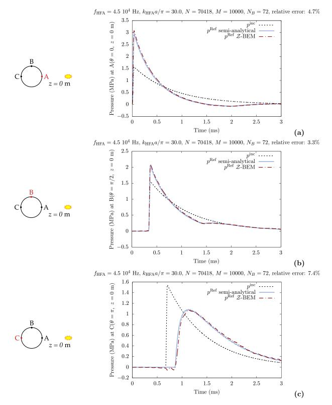
**Figure 6:** Scattering by a small cylinder (a = 0.5 m, L = 5 m, see Fig. 5): comparison between the Z-BEM and semi-analytical solutions for the total field  $p^{\text{Ref}}$  on the z = 0 plane, at the standoff (a), orthogonal (b) and shadow (c) points. The incident field at those points is also shown.
