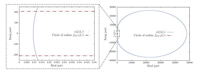
Figure 14: Scattering by a rigid motionless submarine: complex frequencies sL/c used by the Z-BEM. The frequencies for which a BEM problem is solved are concentrated near the origin.
