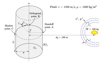
Figure 5: Infinite cylinder facing an underwater explosion.
