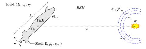
Figure 1: Submarine experiencing a remote underwater blast.
