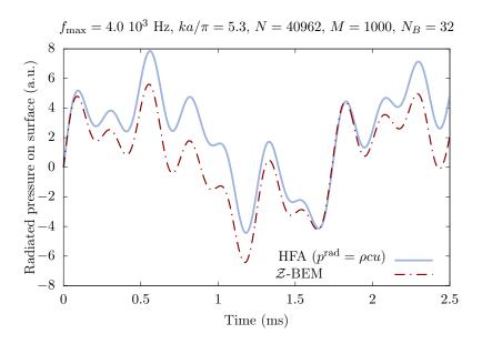
**Figure 4:** Breathing sphere:  $\mathcal{Z}$ -BEM solution and HFA for the radiated pressure  $p^{rad}$  on  $\Gamma$ .
