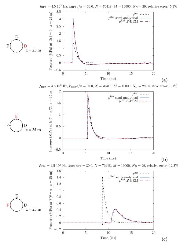
**Figure 9:** Scattering by a large cylinder (a = 5 m, L = 50 m, see Fig. 5): comparison between the Z-BEM and semi-analytical solutions for the total field  $p^{\text{Ref}}$  on the z = 25 m plane, at the standoff (a), orthogonal (b) and shadow (c) points. The incident field at those points is also shown.
