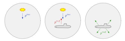
Figure 2: Decomposition of the fluid variables into incident, reflected and radiated parts.
