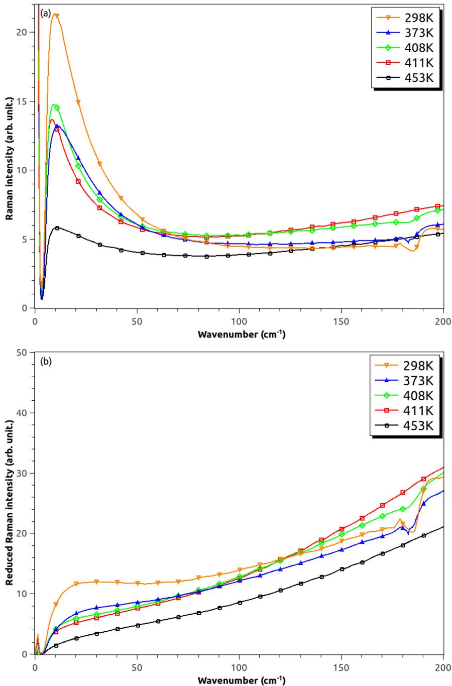
Figure 4. Low- frequency  $Z(XX)\bar{Z}$  Raman spectrum recorded at different temperatures on single  $\text{BaTiO}_3$  crystal: (a) raw data, (b) corrected data according to eq 2.
