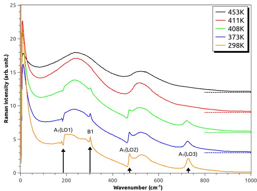
Figure 2. Z(XX)Z Raman spectrum recorded at different temperatures on a single domain BaTiO<sub>3</sub> crystal. The arrows indicate the position of the first-order lines A<sub>1</sub>(LO) and B<sub>1</sub>. The dashed line corresponds to zero intensity line for each temperature.
