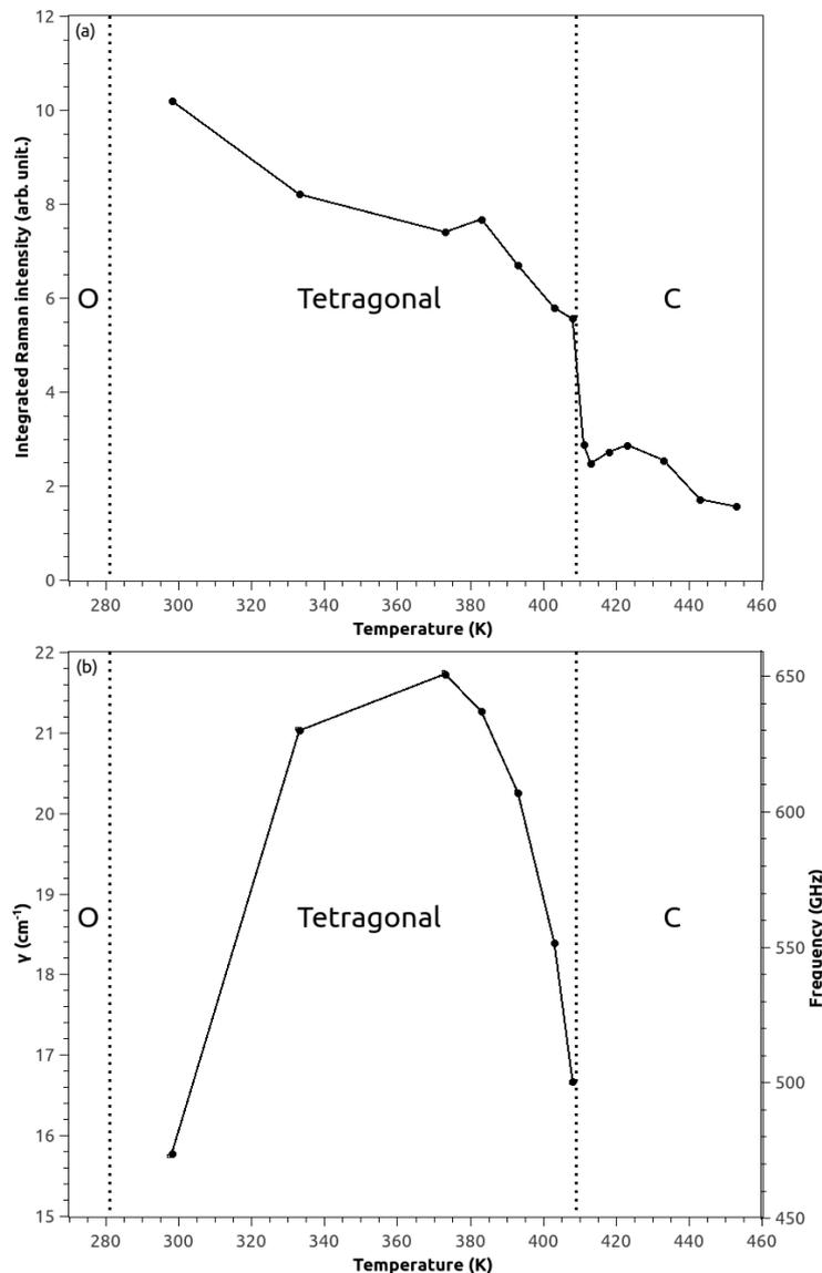
Figure 6. (a) Temperature dependence of the intensity  $J$  integrated between 7 and 100  $\text{cm}^{-1}$  derived from data in fig 5b. (b) Temperature dependence of the inverse relaxation time.
