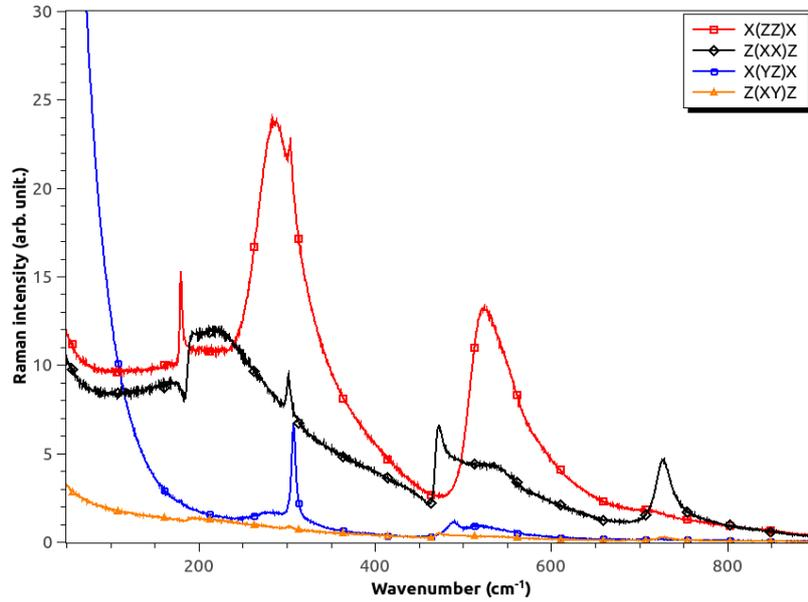
Figure 1. Polarized Raman spectra recorded at room temperature on a single-domain BaTiO<sub>3</sub> crystal.
