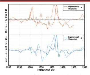
Figure 7. Experimental (-) and wB97X-D/Def2-TZVPP(CHBr<sub>3</sub>) (---) VCD spectra of 7 (top, red) and 9 (bottom, blue), expt first eluted.
