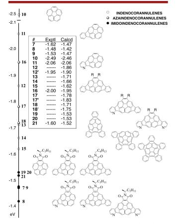
Figure 3. Experimental and B97-D/Def2-TZVPP(THF) first reduction potentials for 7-21. R = H, Me (12, 12', 17, 17', 18, 18').
