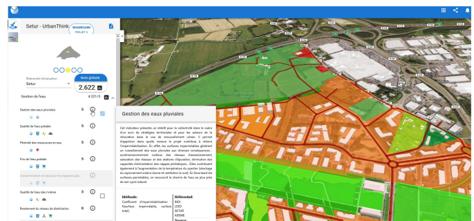
Fig. 12. Example of a rain water management indicator
