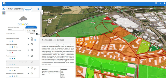
Fig. 12. Example of a rain water management indicator
