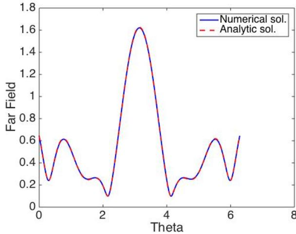
Figure 7: Unit disk. Validation of the code by comparing the analytical and numerical modulus of the far-field for an incident plane P-wave ( $n_{\lambda_s} = 40$  and  $\omega = 2\pi$ ). The  $L^2$  error for this example is  $5.87 \cdot 10^{-3}$ .
