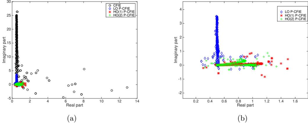
Figure 5: Unit square. Distribution of the eigenvalues of the standard and different P-CFIEs ( $\eta = 1$ ,  $\omega = 2\pi$  and  $n_{\lambda_s} = 20$ ). (a) Complete distribution and (b) closer view of the clustering.
