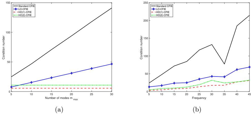
Figure 3: Unit disk. Study of the condition number of the P-CFIEs. (a) Condition number with respect to the maximal number of modes  $m_{\max}$  ( $\kappa_s = 4\pi$ ). (b) Condition number with respect to the frequency ( $n_{\lambda_s} = 12$ ).
