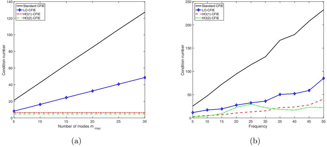
Figure 2: Unit sphere. Study of the condition number of the three P-CFIEs. (a) Condition number with respect to the maximal number of modes  $m_{\max}$  ( $\kappa_s = 4\pi$ ). (b) Condition number with respect to the frequency  $\omega$  ( $n_{\lambda_s} = 12$ ).
