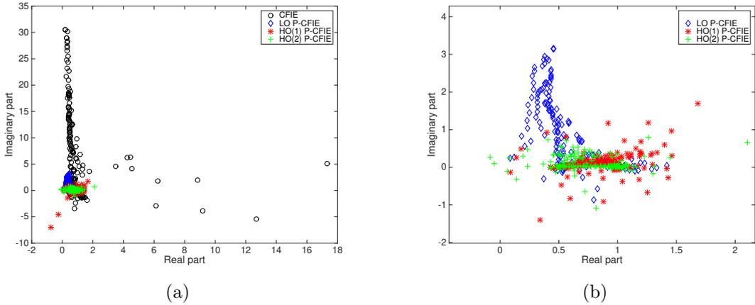
Figure 6: C-shape. Distribution of the eigenvalues of the standard and different P-CFIEs ( $\eta = 1$ ,  $\omega = 2\pi$  and  $n_{\lambda_s} = 20$ ). (a) Complete distribution and (b) closer view of the clustering.
