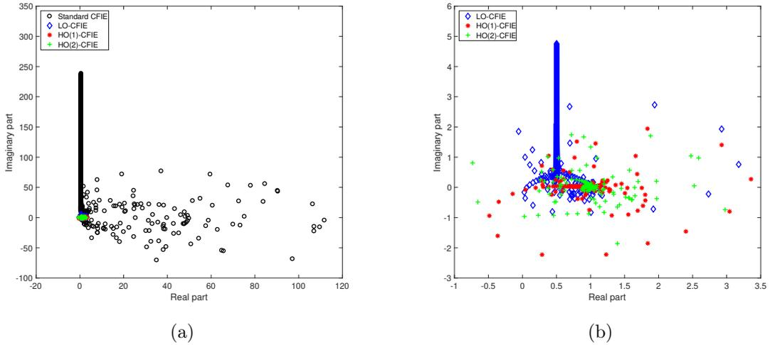
Figure 1: Unit sphere. Distribution of the eigenvalues of the standard and three P-CFIEs ( $\eta = 1$ ,  $\kappa_s = \omega = 50$  and  $n_{\lambda_s} = 12$ ). (a) Complete distribution and (b) Closer view on the clustering.
