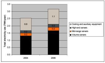
Figure 4: Total electric use for servers in France in 2004 and 2006, including cooling and auxiliary equipments
