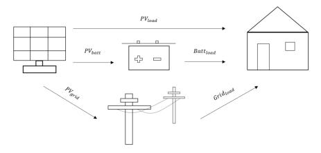
Figure 2: Electric flow chart of the PV-battery installation
