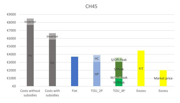
Figure 10: Breakdown of the costs and incomes from a 3 kW PV (W: Winter; S: Summer)
