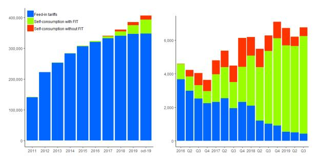
Figure 1: Cumulated PV up to 36 kW (left) and quarterly evolution (right) in France – Source : Enedis (2018)¹
