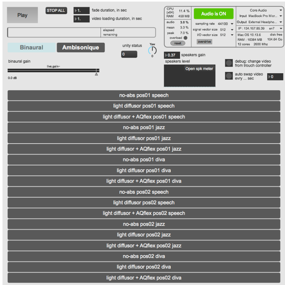
Figure 4: Max Presentation Patch: enables to instantly toggle the sound reproduction system ( Ambisonic or Binaural ), the position in the Atrium ( close or farther ), the acoustical treatment , and adjust volume .
