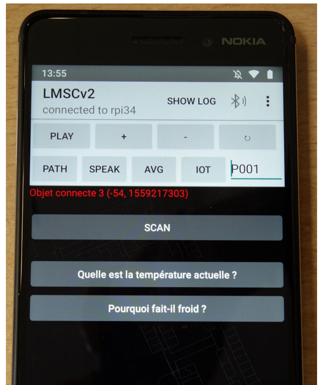
FIGURE 13. Display of some available queries, in French (a: What is the current temperature? b: Why is it cold?) on the SO2SEES smartphone application.
