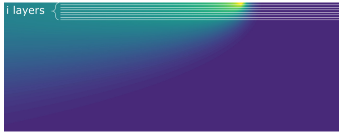
(a) Thermal field during the printing of layer i .
