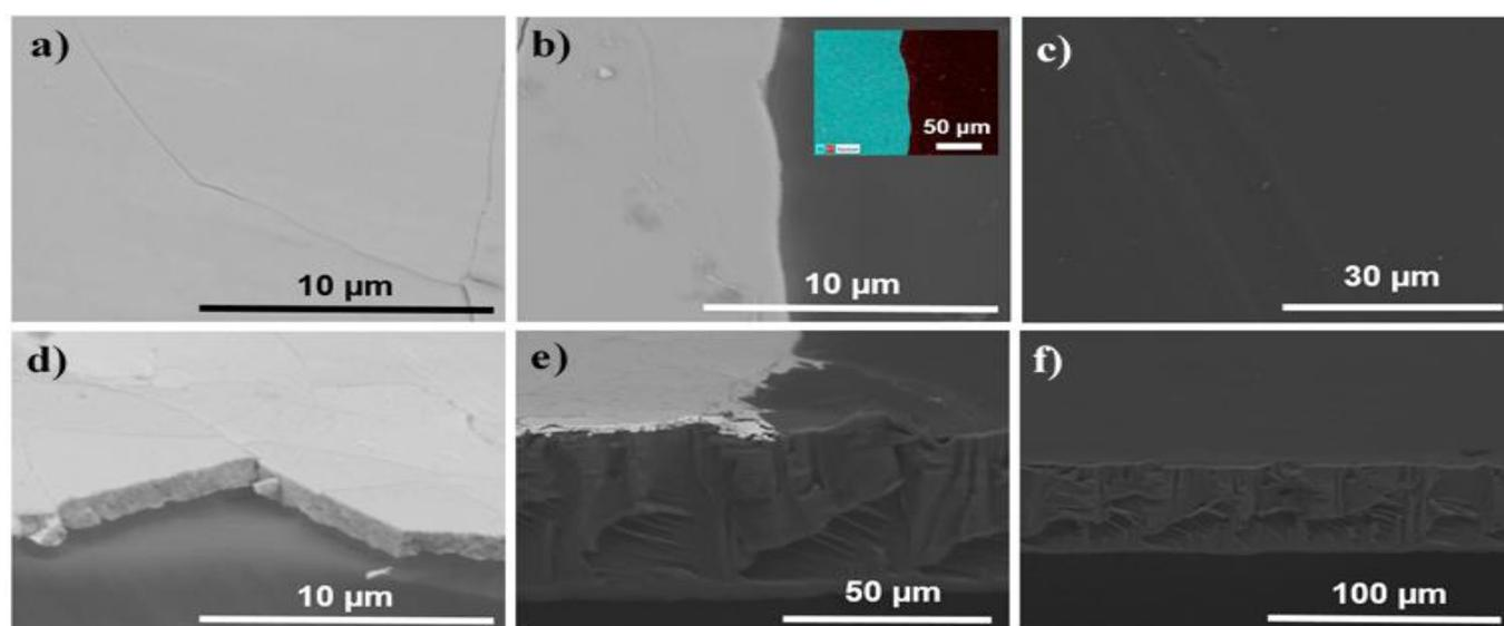
Fig. 1 SEM images of the hybrid chiral imprinted Pt-PPy film at different positions. (a,d) top and side view of the chiral-encoded platinum layer, (b, e) top and side view of the Pt-PPy junction (inset: EDS map), (c,f) top and side view of the PPy film.
