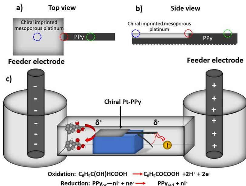
Scheme 1. Illustration of the hybrid Pt-PPy film used for chiral recognition (a) Top view and (b) cross section of Pt-PPy (c) Scheme of the bipolar electrochemical cell for chiral recognition of mandelic acid with the hybrid actuator.
