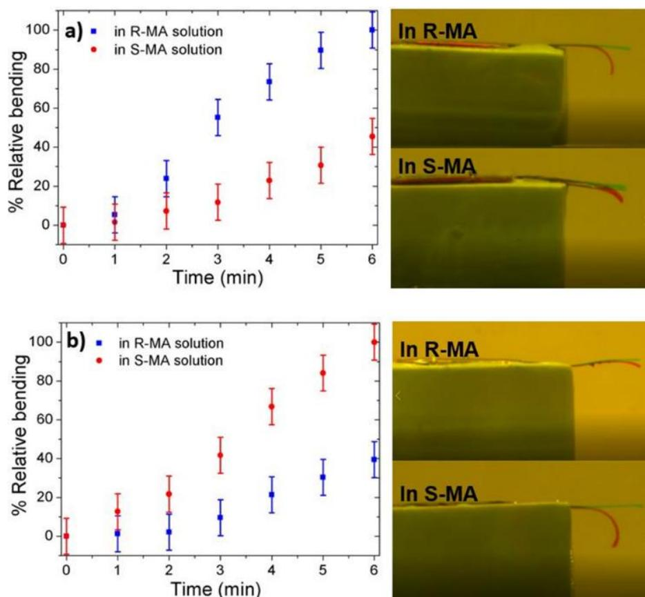
Fig. 2 Bipolar electrochemical actuation of hybrid chiral Pt-PPy in 50 mM R-MA (blue) and S-MA (red) using 50 mM HCl as supporting electrolyte. Relative bending measured as a function of time for (a) R-MA imprinted Pt-PPy and (b) S-MA imprinted Pt-PPy. The pictures on the right have been taken after 6 min of applied potential. The green line indicates the initial position of the actuator, whereas red corresponds to its final position.
