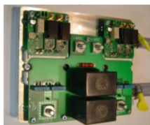
Fig. 8 Photos of the fabricated wireless charger (a) Fabricated coupler, (b) Fabricated primary inverter
