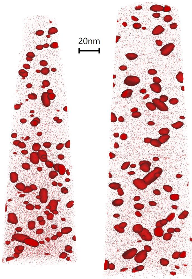
Figure 3: APT reconstructions of the as-received (left) and aged 15000h@350°C (right) where are displayed 10at% Cu isoconcentration surfaces (Cu precipitates) together with 25% of the total Cu atoms.
