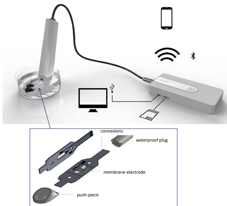
Figure 10: Photograph of the prototype showing, immersed in a 125mL glass beaker container, a support holding the membrane-electrode pad. Membrane-electrode pads are connected to the measurement device via the support cable -inset: pad components, the membrane-electrode is sandwiched in middle where the open windows allow a permanent contact with the electrolyte. A dedicated software drives the overall system.
