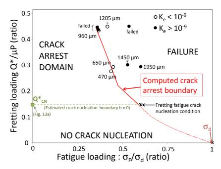
Fig. 14. Computed crack arrest fretting fatigue map.
