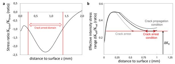
Fig. 12. (a) R<sub>k</sub> stress ratio along the crack path; (b) crack arrest condition determination.
