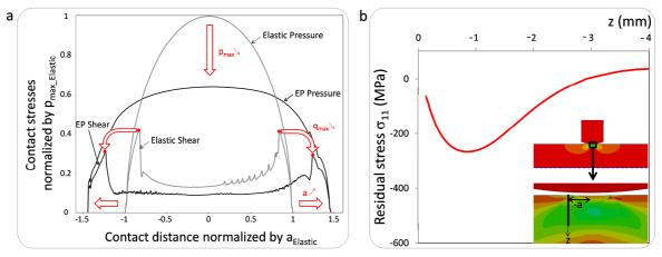
Fig. 9. (a) Contact stresses; (b) Distribution of the  $\sigma_{11}$  residual stress (after the contact opening) ( $\sigma_F/\sigma_d = 0.435$ ,  $Q^*/\mu P = 0.294$ )
