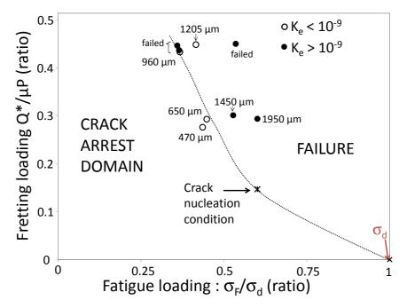
Fig. 6. Crack arrest experimental fretting-fatigue map
