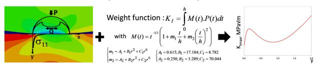
Fig. 10. Stress extraction along crack path for a fretting fatigue case.
