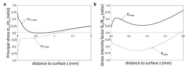
Fig. 11. (a) Principal stress at the contact border; (b) Stress intensity factors at the contact border
