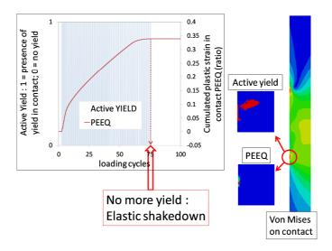
Fig.8. Monitoring of the elastic shakedown on contact.
