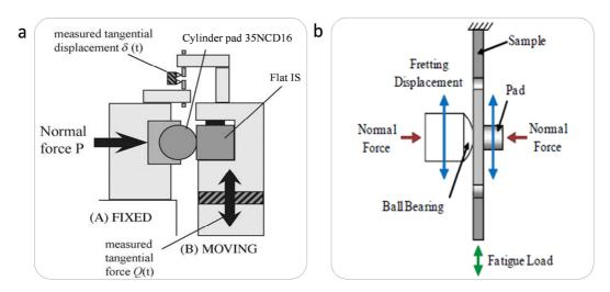
Fig. 2. (a) Plain fretting test; (b) Fretting-fatigue test.
