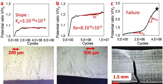
Fig. 5. (a) Crack arrest condition; (b) Crack propagation condition; (c) Failure condition. Vo: potential measured at the test beginning
