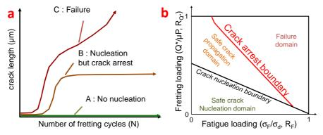
Fig. 1. (a) Crack nucleation and propagation in fretting-fatigue; (b) Fretting fatigue map.
