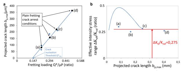
Fig. 13. (a) Plain fretting experimental results; (b) Crack arrest condition identification on plain fretting conditions (P, 10<sup>6</sup> cycles, 12 Hz)
