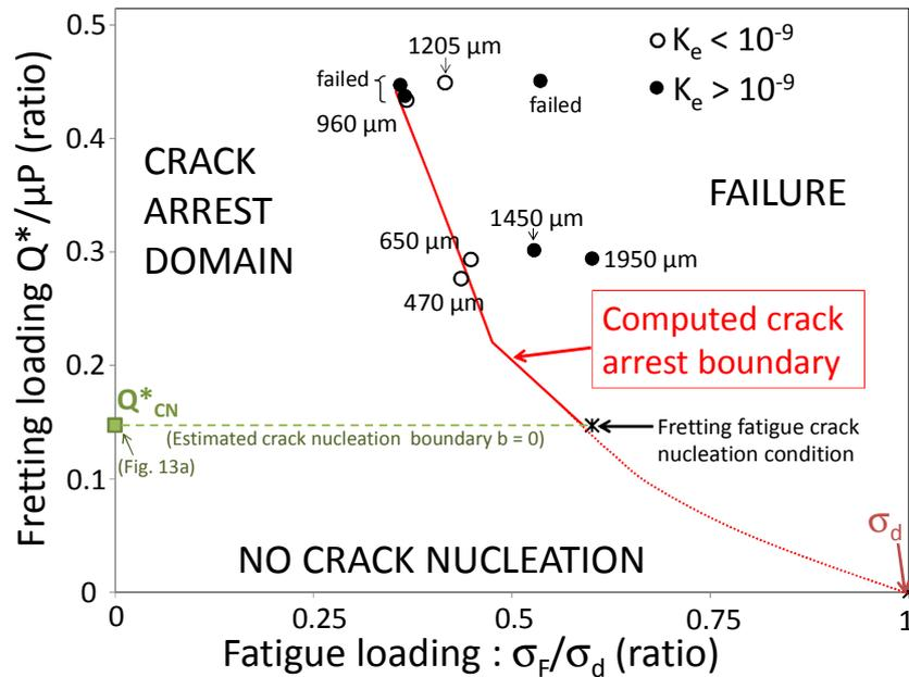
Fig. 14. Computed crack arrest fretting fatigue map.
