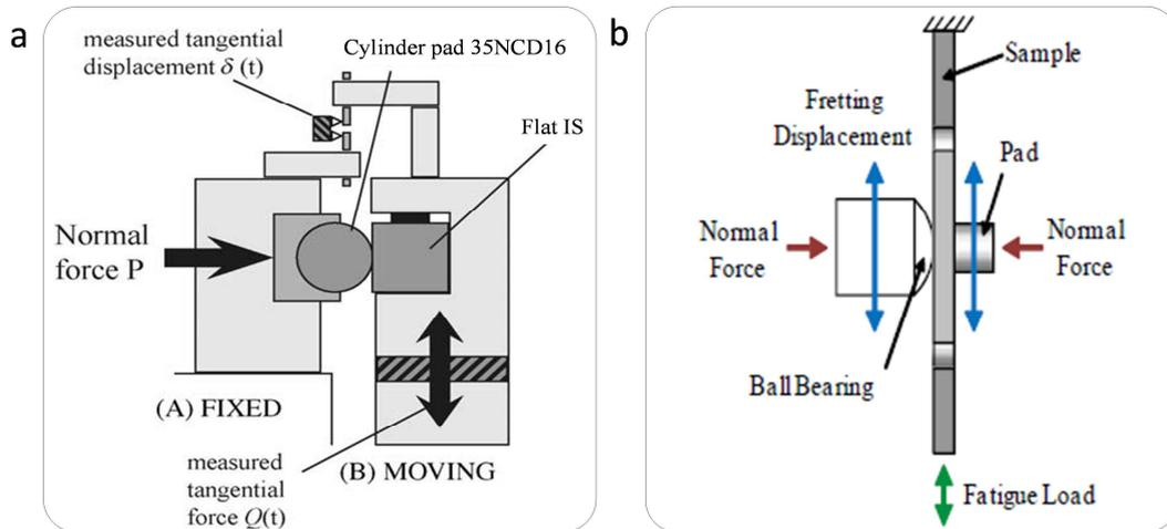
Fig. 2. (a) Plain fretting test; (b) Fretting-fatigue test.
