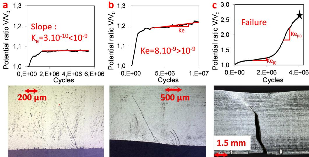
Fig. 5. (a) Crack arrest condition; (b) Crack propagation condition; (c) Failure condition.  $V_0$ : potential measured at the test beginning
