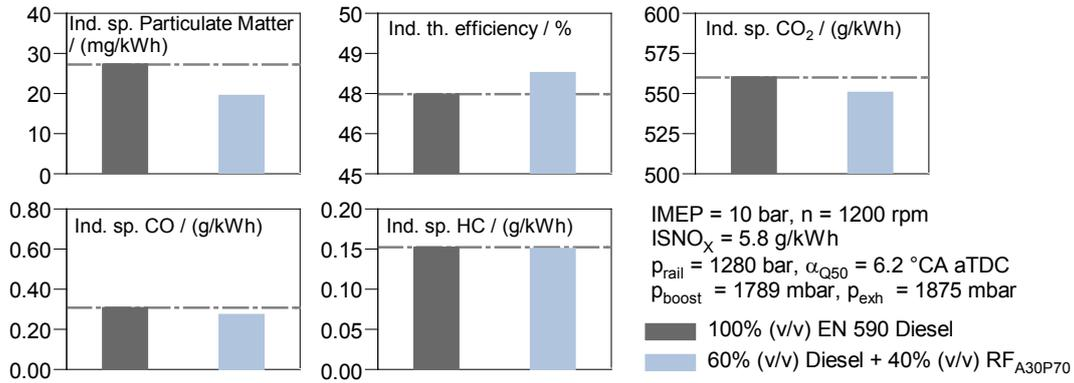
Figure 8. Engine test results of EN590 diesel and the blend of 60% (v/v) diesel and 40% (v/v) RF<sub>A30P70</sub> at n = 1200 rpm and IMEP = 10bar
