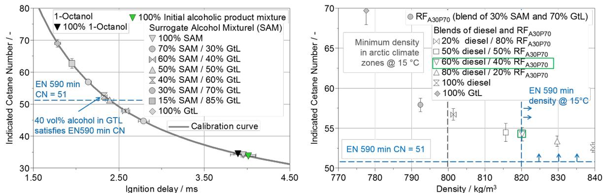
Figure 4: Indicated Cetane Number determination of Surrogate Alcoholic Fuel (SAF), real product mixture and blends of SAF and GtL (ref. 2, left panel), Indicated Cetane Number v/s density graph for different blends of REDIFUEL (ref. 2, right panel)
