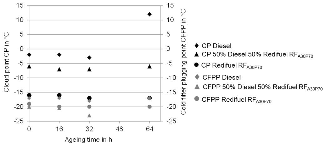
Figure 5. Cold Properties of diesel, RF<sub>A30P70</sub> and a blend of 50% (v/v) diesel and 50% (v/v) RF<sub>A30P70</sub>
