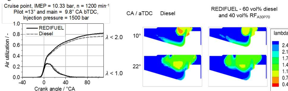
Figure 7: Comparison of Air utilization (ref. 3, left), and lambda plots for RF<sub>A30P70</sub> and diesel (ref. 3, right), at cruise power point
