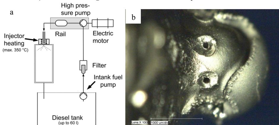
Figure 6: (a) General setup of one of the 4 test places at the “ENIAK” CoCoS test bench (Hoffmann, 2018); (b) External deposits after test run (1,300 bar, 10 Hz, 500  $\mu$ s, B10 with performance additive) (Hoffmann et al, 2015)
