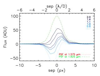
**Fig. 5.** Radial profiles of residual SDI patterns along the shift direction, separated by  $6\lambda/D$  (300 mas) from the center of the image. PSF profiles are overplotted (dashed and dotted lines). The legend value indicates F1/F3 (and corresponds to F3/F1 = 0.5, 0.8, 0.9, 1.0, 1.2, and 1.5). All profiles have been centered on 0 for clarity.
