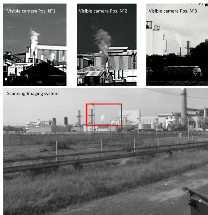
Figure 5. The different raw images at the same time of the 3 visible cameras (GoPro Hero3 with zoom) and the scanning imaging system (SIGIS Bruker without zoom) during the measurements. The infrared measurement grid is also indicated (red rectangle).
