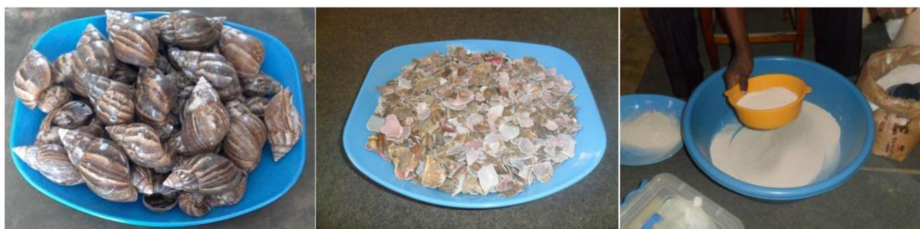
**Fig. 1** Photos of some steps of powdering snail shells
