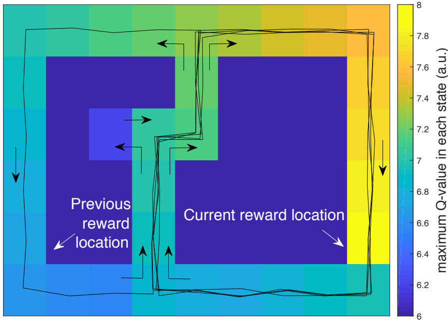
Fig. 3 Example of Q-values learned by the model during simulations of a simplified version of the multiple T-maze task of Gupta et al. (2010). The color code illustrates the gradient of Q-values learned at the end of the experiment, when the reward is located in the right arm. The continuous black line represents the trajectories (noised for illustrative purpose) performed by the agent during the last six trials of the experiment. Black arrows indicate the directions that are allowed to the agent during task performance. The two states in the central arm where the agent has the choice to go either left or right are called the decision points throughout the manuscript. The agent is not allowed to immediately get back to the state visited at the previous timestep, except for the state located at the left of the central decision-point, where the only possibility is to move towards the east. The small Q-values in dark blue correspond to areas of the maze unreachable by the agent, due to the corridors’ walls. They thus remain unchanged during the experiment.
