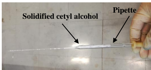
Figure 10. Cetyl alcohol solidified in the pipette after 30 seconds
