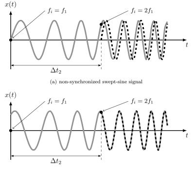
(b) synchronized swept-sine signal starting with a non-zero phase
