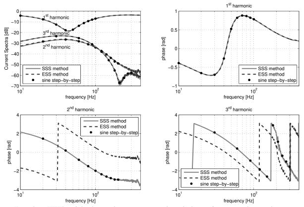
**Figure 7.** First three HHFRs of the distorted current passing through the woofer estimated using the non-synchronized swept-sine signal ESS (dashed line) and the synchronized swept-sine signal SSS (gray line), compared with a step-by-step measurement using a sine-wave excitation (dots).
