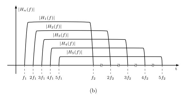
**Figure 6.** Schematic representation of magnitude spectra of HHFRs  $H_n(f)$ . (a) The deconvolution using Eqs. (4) or (7) set the upper bandwidth limit to  $f_2$ . (b) The deconvolution using the analytic expression in Eq. (38) does not limit the frequency bandwidth of HHFRs.
