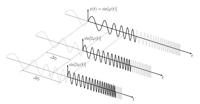
**Figure 3.** Delaying the Synchronized swept-sine signal  $x(t) = \sin[\varphi(t)]$  by  $\Delta t_2$  and by  $\Delta t_3$  is equivalent to generating the second and third harmonic  $\sin[2\varphi(t)]$  and  $\sin[3\varphi(t)]$  of the Synchronized swept-sine signal x(t).
