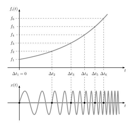
**Figure 4.** Synchronized swept-sine x(t) (below) and the associated instantaneous frequency  $f_i(t)$ .
