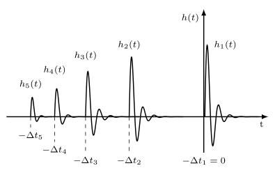
**Figure 5.** Result of the deconvolution process resulting in a sum of time-shifted higher harmonic impulse responses  $h_n(t)$
