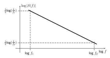
Figure 5. Amplitude of the Fourier Transform of the exponential swept-sine signal.
