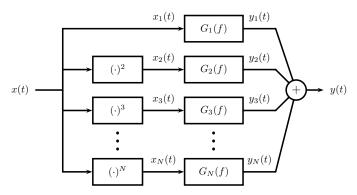
Figure 1. Generalized Polynomial Hammerstein model (power series nonlinear model).
