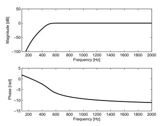
Figure 7. The theoretical frequency response (modulus - above; phase - below) of the filter  $G_1(f)$  from the linear part of the tested system.
