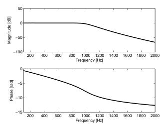
Figure 9. The theoretical frequency response (modulus - above; phase - below) of the filter  $G_3(f)$  from the nonlinear part of the tested system.
