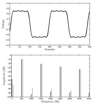
Figure 12. Comparison of the real-world (thin) and regenerated (bold) responses (waveforms - left; spectra - right) to the sine-wave f = 500Hz, A = 1V.
