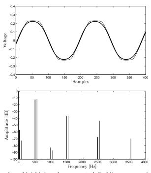
Figure 13. Comparison of the real-world (thin) and regenerated (bold) responses (waveforms - left; spectra - right) to the sine-wave f = 500Hz, A = 0.3V.
