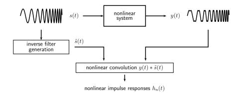
Figure 2. Block diagram of the nonlinear convolution process in NLS identification.
