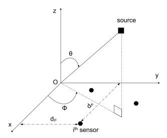
Fig. 1. 3D source localization using a planar array.
