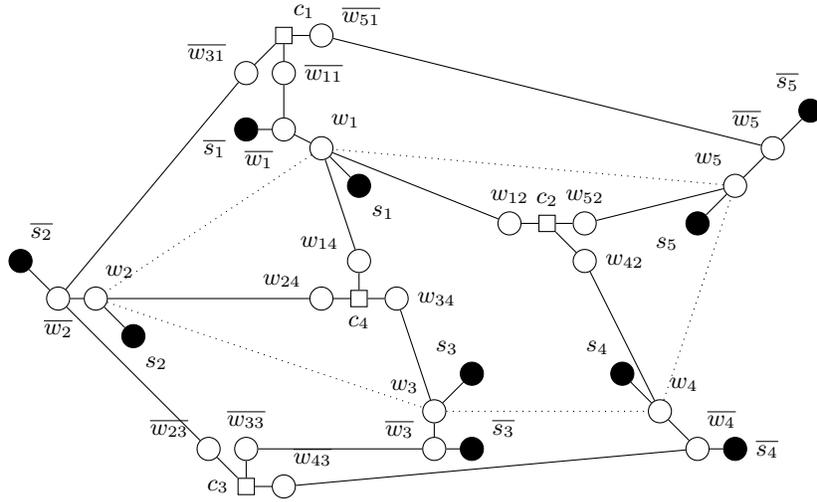
**Fig. 2.** Reduction from the instance of Figure 1 to an instance of the WDA-VALID problem. Switches, consumers and sources are respectively circles, rectangles and filled circles. The dotted lines represent the variable cycle which is deleted at step 2.
