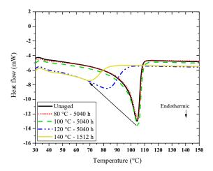
Figure 4. DSC heating thermograms of XLPE samples before and after thermal aging at  $80,\,100,\,120$  and  $140\,^{\circ}\text{C}$ .
