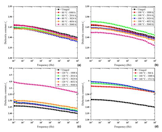
Figure 6. Variation of the dielectric constant of XLPE samples versus frequency at aging temperatures of: (a) 80 °C, (b) 100 °C, (c) 120 °C and (d) 140 °C, for different durations.
