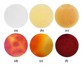
**Figure 1.** Color change of XLPE samples: (a) before aging, (b) aged at  $80 \,^{\circ}$ C for 5040 h, (c) aged at  $100 \,^{\circ}$ C for 5040 h, (d) aged at  $120 \,^{\circ}$ C for 5040 h, (e) aged at  $140 \,^{\circ}$ C for 504 h, (e) aged at  $140 \,^{\circ}$ C for  $1512 \,^{\circ}$ h
