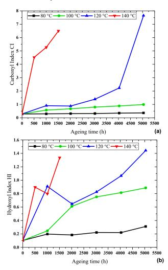
**Figure 3.** Evolution of (a) Carbonyl index and (b) Hydroxyl index, versus aging time.
