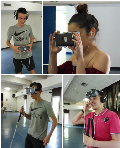
Fig. 5. Ways of wearing the VR system: (top left) hand-held without seeing the screen, (top right) hand-held seeing the screen, (bottom left) head-worn in front of his eyes, and (bottom right) on forehead.
