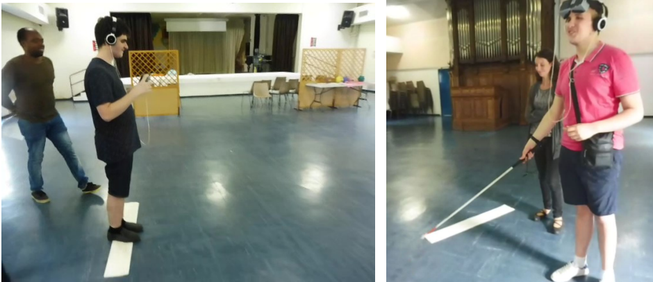
Fig. 3. Physical tactile paving aligned with the virtual pedestrian crossing. In the virtual world, the student is in front of the virtual pedestrian crossing, on the sidewalk and at 50 cm of the road.
