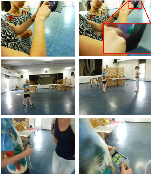
Fig. 8. Top left: The instructor touches the screen to position the virtual cube anywhere in the room. Top right: when touching the screen, a green cube is instantiated in the environment. Middle left: a student follows spatial audio feedback depending on his/her position relative to the cube. Middle right: the student identifies the cube's position. Bottom left: the student shows the teacher the screen for verification. Bottom right: the cube is visible in the screen, i.e. the position is correct.
