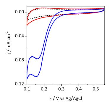
Figure 7: CVs of *Tt* Lac C445A adsorbed on Neg-CNT in the absence (black dashed line) and presence (red line) of 1 mM CuSO<sub>4</sub>. The blue line represents the CV for Neg-CNT with *Tt* Lac WT in the presence of 1 mM CuSO<sub>4</sub>. 0.1 M NaAc buffer pH 5, scan rate 5 mV s<sup>-1</sup>, O<sub>2</sub> atmosphere.
