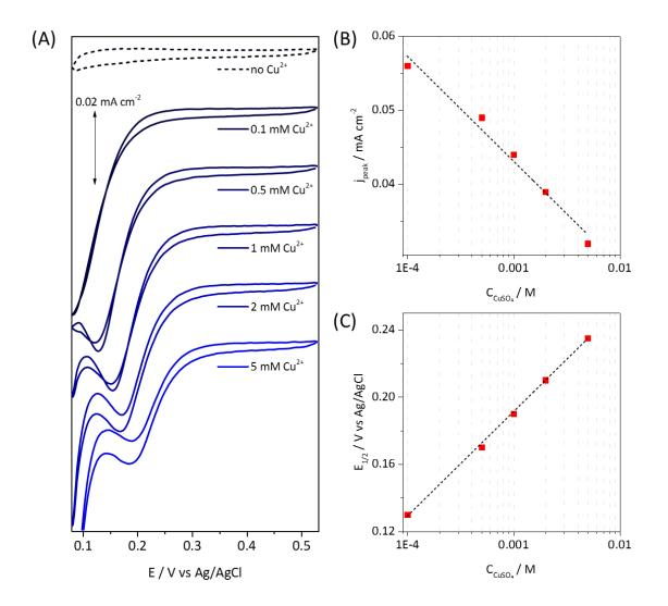
Figure 6: (A) CVs under O<sub>2</sub> with *Tt* Lac adsorbed on Neg-CNT in the presence of increasing CuSO<sub>4</sub> concentrations from zero to 5 mM. (B, C) Dependence of the half wave potential and peak current density on CuSO<sub>4</sub> concentration. 0.1 M NaAc buffer pH 5, scan rate 5 mV s<sup>-1</sup>.
