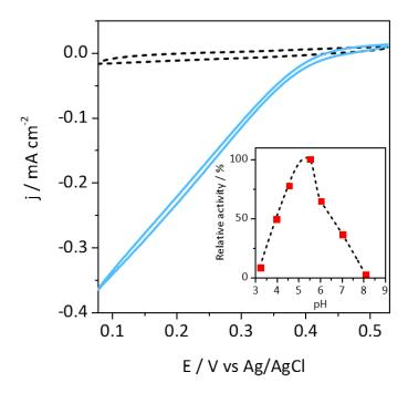
Figure 3: CVs at Pos-CNT in the presence of Tt Lac under  $O_2$  (blue line) or  $N_2$  (black dashed line). Electrode rotation speed 800 rpm, scan rate 5 mV s<sup>-1</sup>. Inset: Relationship between Tt Lac relative activity and pH for  $O_2$  catalytic reduction at the Pos-CNT.
