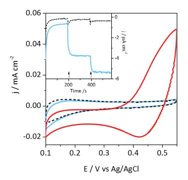
Figure 4: CVs for  $O_2$  reduction on Neg-CNT in the absence of Tt Lac (black dashed line), in the presence of Tt Lac (blue solid line) and in the presence of Tt Lac and 1 mM ABTS (red solid line). 0.1 M NaAc buffer pH 5, scan rate 5 mV s<sup>-1</sup>. Inset: chronoamperometry of  $O_2$  reduction at 0.2 V in the absence (black dashed line) and in the presence of Tt Lac (blue solid line); 1 mM ABTS was added at 200 s and 400 s as indicated by arrows.
