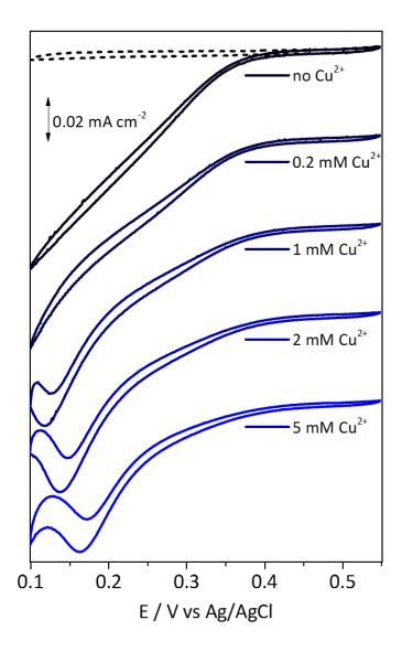
Figure 8: CV responses under  $O_2$  by Tt Lac adsorbed on Pos-CNT with increasing concentrations of CuSO<sub>4</sub> from 0 to 5 mM. Dashed curve represents the same electrode in the absence of CuSO<sub>4</sub> under  $N_2$ .
