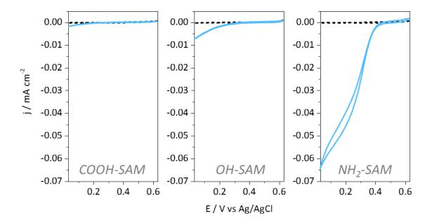
Figure 2: CV responses of O<sub>2</sub> reduction by *Tt* Lac adsorbed on different SAM-modified gold electrodes: 6-MHA (COOH-SAM), MH (OH-SAM), and CYST (NH<sub>2</sub>-SAM). Dashed lines represent SAM-modified gold electrodes without *Tt* Lac. 0.1 M NaAc buffer pH 5, scan rate 5 mV s<sup>-1</sup>.
