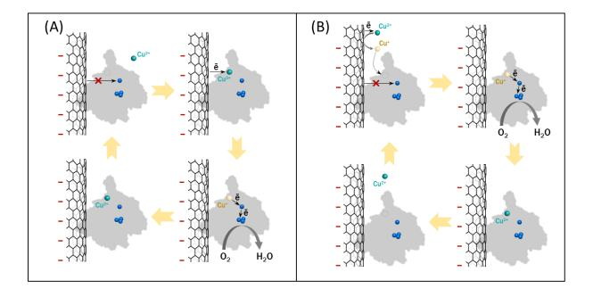
Scheme 1. Proposed mechanisms of copper-induced catalytic wave formation on Neg-CNTs-*Tt* Lac: (A) copper – electron relay according to the hypothesis iii and (B) copper – substrate according to the hypothesis iv.
