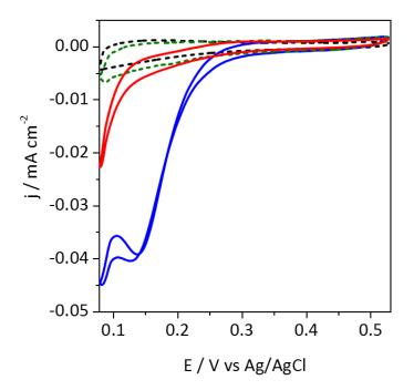
Figure 5: CVs under  $O_2$  of Tt Lac adsorbed on Neg-CNT without (black dashed curve) or in the presence of 500  $\mu$ M CuSO<sub>4</sub> (blue solid curve). CV under  $N_2$  of Tt Lac adsorbed on Neg-CNT in the presence of 500  $\mu$ M CuSO<sub>4</sub> is given as a green dashed curve. The red curve is obtained after 40 mM NaF addition in the oxygenated buffer containing CuSO<sub>4</sub>. 0.1 M NaAc buffer pH 5, scan rate 5 mV s<sup>-1</sup>.
