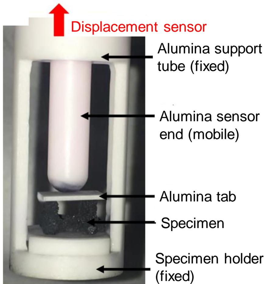
SupMat 4: Close view of thermomechanical device used for the thermal strain thermal expansion coefficient measurements (Fig. 16)
