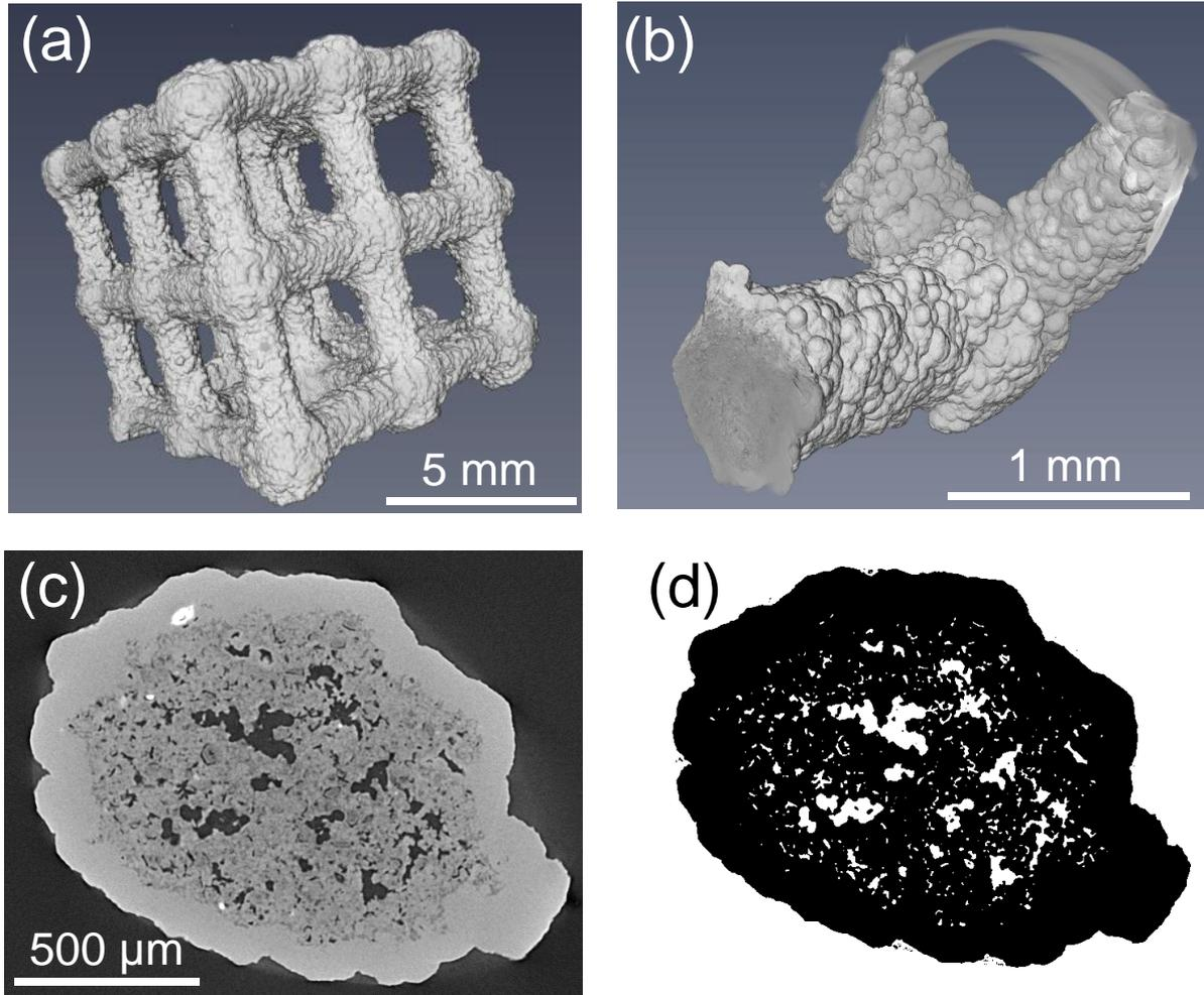
Fig. 10. X-ray tomography images of the CVI/CVD lattice structure: (a) overall perspective view obtained at low resolution ( $23\ \mu\text{m}$ ), (b) perspective view at high resolution ( $2\ \mu\text{m}$ ) of a node and its neighboring struts, (c) example of a greyscale image of a strut cross-section, (d) equivalent threshold image
