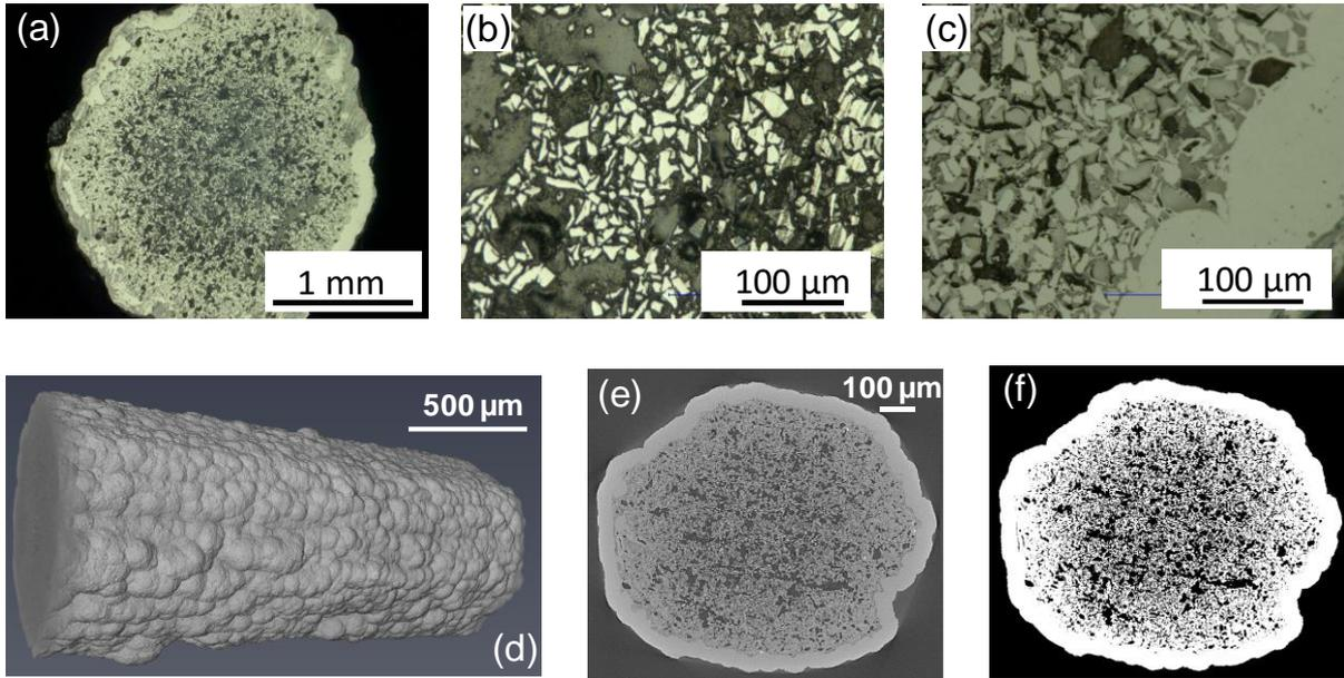
SupMat 5: Cross-section of a rod after CVD, as examined by optical microscopy (overall section (a), core region (b), near surface region (c)) and X-ray tomography (overall perspective view (d), greyscale image of the cross-section (e), equivalent threshold image (f))
