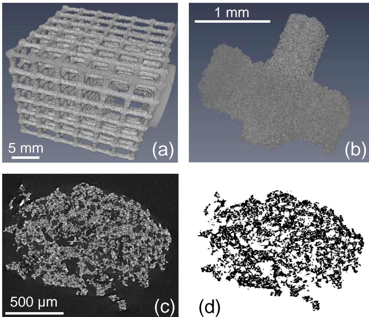
Fig. 9. X-ray tomography images of the PIP lattice structure: (a) overall perspective view obtained at low resolution ( $23\ \mu\text{m}$ ), (b) perspective view at high resolution ( $2\ \mu\text{m}$ ) of a node and its neighboring struts, (c) example of a greyscale image of a strut cross-section, (d) equivalent threshold image
