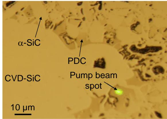
Fig. 16. Optical microscope image of a cross-section of a CVI/CVD lattice structure showing the different SiC-based components and the pump beam spot focused on a PDC part. The darkest zones correspond to pores, brown regions to PDC areas and lightest zones to  $\alpha$ -SiC particles and the CVD-SiC coating
