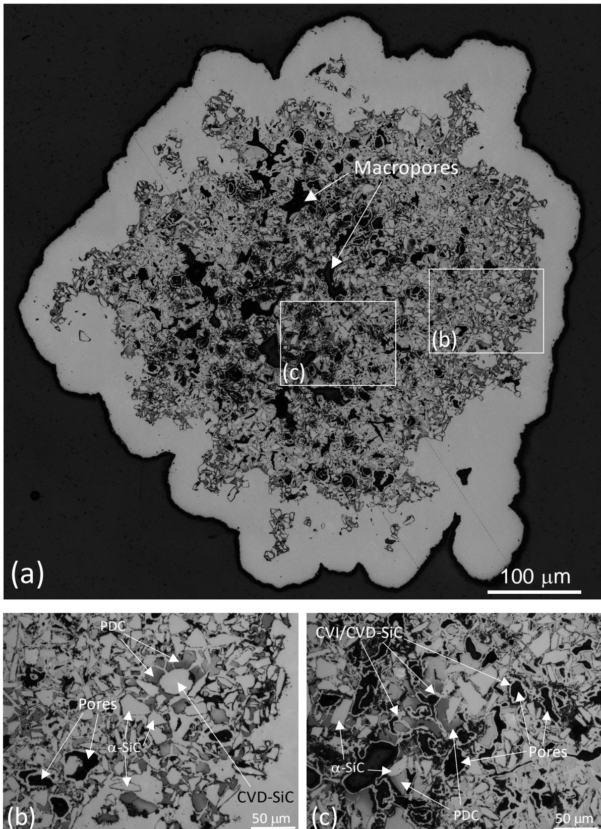
Fig. 7. Strut cross-section of a in a CVI/CVD lattice structure: (a) overview, (b) close view near the surface, (c) close view of the core
