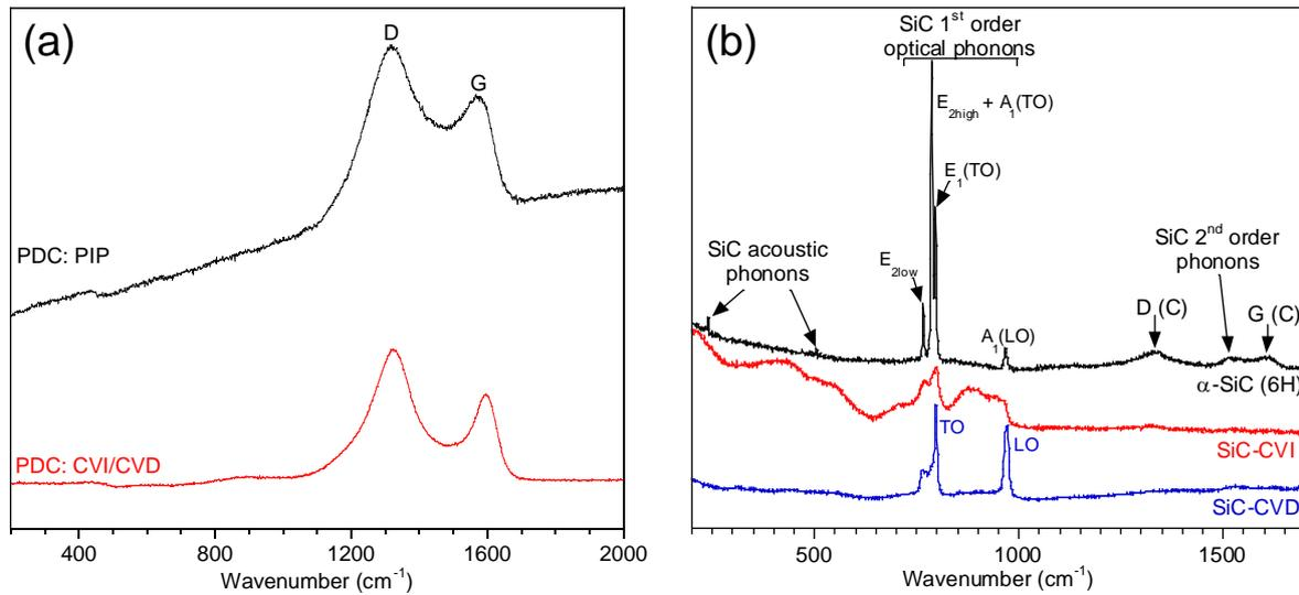
Fig. 5. (a) Raman spectra of the PDC parts in the lattice structures at various stages of the process, (b) Raman spectra of an  $\alpha$ -SiC particle, the CVI and the CVD-SiC coating in the lattice structures
