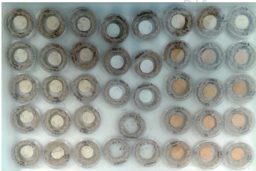
247 Figure 2: Termite screening test set-ups at the start of termite exposure.
