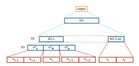
Figure 3: MLP-MS architecture for ASR error detection task, that integrates signal and acoustic word embeddings in addition to the baseline features.
