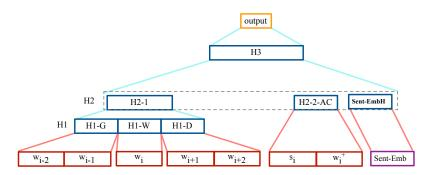
Figure 4: MLP-MS architecture for ASR error detection task, that integrates acoustic and sentence embeddings in addition to the baseline features.
