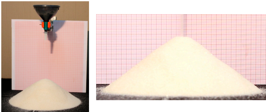
Figure 1. Illustration of sand pile growth (right) and description of the apparatus used to measure the heap height (left).
