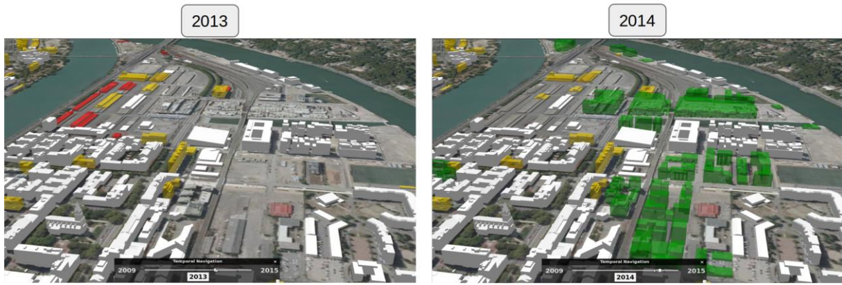
Figure 11. Screenshots showing the evolution of a district of the city of Lyon (in 2013 on the left side and in 2014 on the right side) visualized in UD-Viz and using 3D Tiles extended with 3DTiles_temporal .
