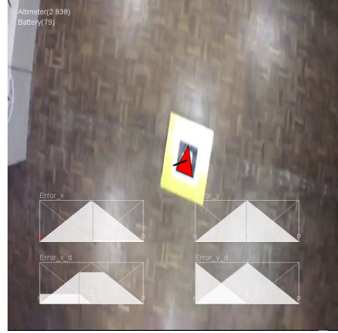
Fig. 11. The FLC membership functions overview on the GUI
