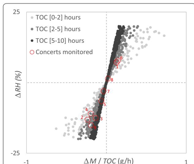
**Fig. 6** Simulation of 1000 concerts using randomly sorted environmental conditions in the range of  $-20\% < \Delta RH < 20\%$  and  $0.5 \text{ h} < TOC < 10 \text{ h}$
