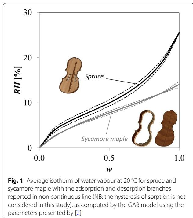
**Fig. 1** Average isotherm of water vapour at 20 °C for spruce and sycamore maple with the adsorption and desorption branches reported in non continuous line (NB: the hysteresis of sorption is not considered in this study), as computed by the GAB model using the parameters presented by [2]
