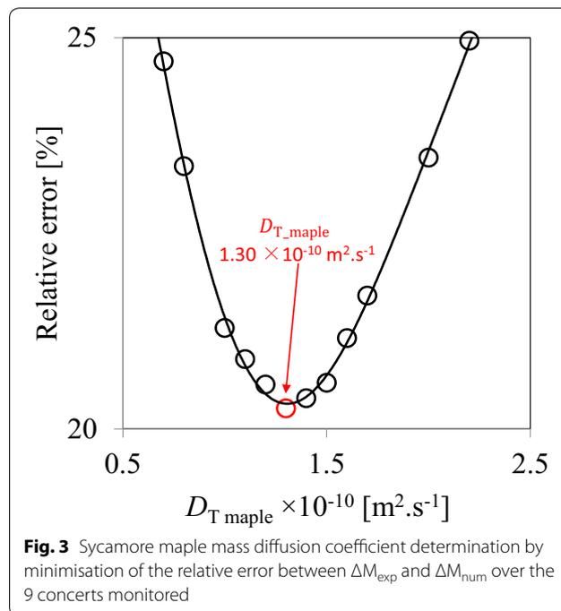
**Fig. 3** Sycamore maple mass diffusion coefficient determination by minimisation of the relative error between  $\Delta M_{exp}$  and  $\Delta M_{num}$  over the 9 concerts monitored
