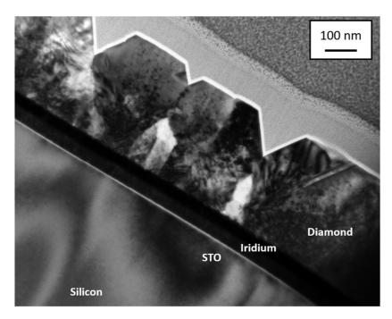
Figure 6 TEM bright field image of the full stacking of the diamond/Ir/STO/Si (001) sample
