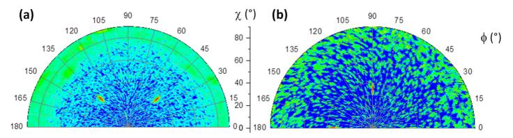
**Figure 10** XRD half pole figures around (a) the (111) reflection of the diamond layer; (b) the (111) reflection of the silicon substrate.
