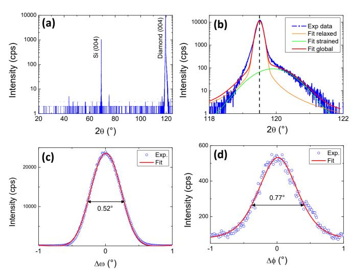
**Figure 8** XRD characterization of epitaxial diamond layer grown on Ir/STO/Si(001): (a) large  $\theta/2\theta$  scan; (b)  $\theta/2\theta$  scan focused on the (004) reflection of diamond; (c)  $\omega$ -scan around the (004) reflection of the diamond; (d)  $\phi$ -scan around the (220) reflection of the diamond at the surface region in GIXRD.
