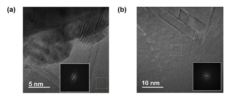
**Figure 7** HRTEM bright field images taken along the <110> zone axis (a) at the diamond/Ir interface; (b) inside the diamond film at 100 nm from the diamond/Ir interface. Inserts showed FFT extracted from the squared area indicated with red dotted lines.
