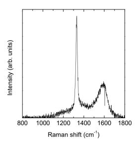
**Figure 5** Raman spectrum of the 310 nm-thick diamond heteroepitaxial layer grown on Ir/STO/Si (100). UV laser excitation at 325 nm.
