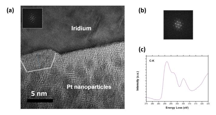
**Figure 4** (a) HRTEM bright field image of a diamond nanocrystal at the surface of the Ir monocrystalline epilayer which underwent the BEN step. This nanocrystal is identified by a white contour; Platinum nanoparticles from the protective coating are observed on the HRTEM image. (b) Fast Fourier Transform of the HRTEM image of the diamond nanocrystal; (c) C-K EELS spectrum recorded on such a nanocrystal.
