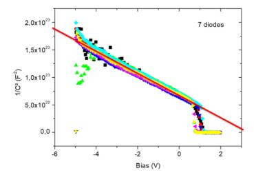
Figure 15: 1/C<sup>2</sup> - V curves of 7 diodes from all over the sample and in red the linear fit
