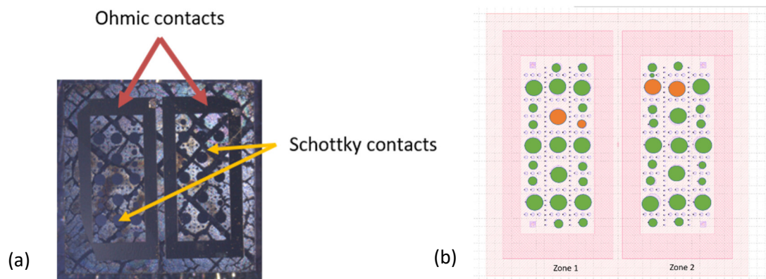
Figure 13 a) Optical image of the final device. Note that the cracks are located on the backside of the diamond crystal and seen by transparency (see details in the text); b) Mapping of the devices that present a diode behavior with rectification (in green) or (in orange) no rectification
