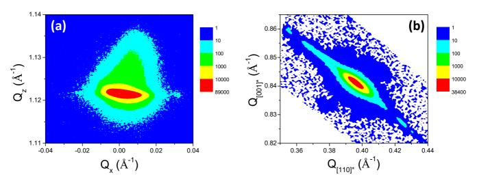
**Figure 9** XRD reciprocal space maps from the epitaxial diamond layer on Ir/STO/Si(001) around (a) the (004) node, and (b) the (113) node.
