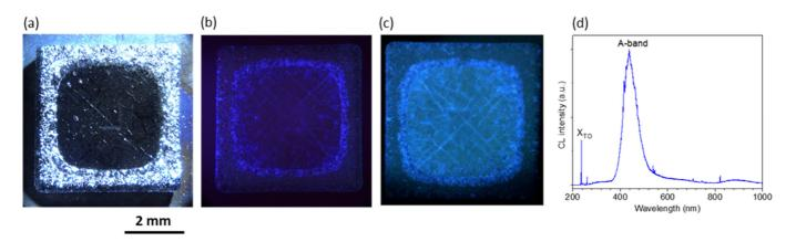
**Figure 11** (a) Optical image of the thick diamond film grown on Ir/STO/Si (001) substrate. Besides are shown luminescence images in the visible range at 300K; (b) CL and (c) DiamondView<sup>TM</sup>; (d) Typical CL spectrum taken at 10 K on the final growth surface in the 200-1000 nm range.
