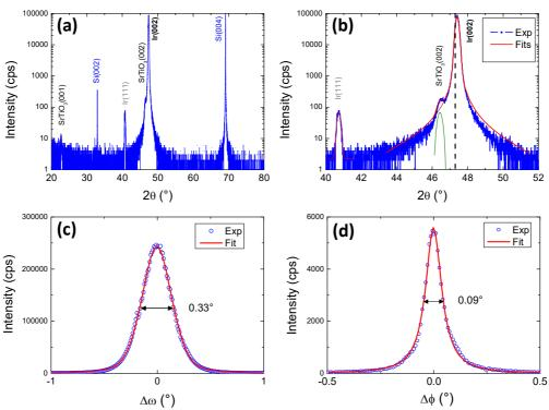
**Figure 2**: XRD characterization of Ir/STO/Si(001) heterostructure: (a) large  $\theta/2\theta$  scan, (b)  $\theta/2\theta$  scan focused on the (111)<sub>Ir</sub> and (002)<sub>Ir</sub> reflections (vertical black dashed line indicates the position of the bulk Ir(002) reflection), (c) ω-scan around the (002)<sub>Ir</sub> reflection, (d) φ-scan around the (200)<sub>Ir</sub> reflection at the surface region in grazing incidence configuration (GIXRD).
