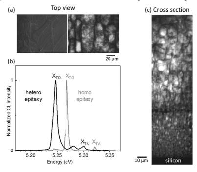
**Figure 12** (a) SEM and CL images of free exciton recombination ( $X_{TO}$  filtered at 235 +/- 3 nm) recorded from the surface; (b) Typical CL spectrum in the UV range observed at the surface, compared with a commercial homoepitaxial diamond layer (Element 6 electronic grade); (c) CL image of free exciton recombination ( $X_{TO}$  filtered at 235 +/- 3 nm) of the cross-section of the heteroepitaxial layer.
