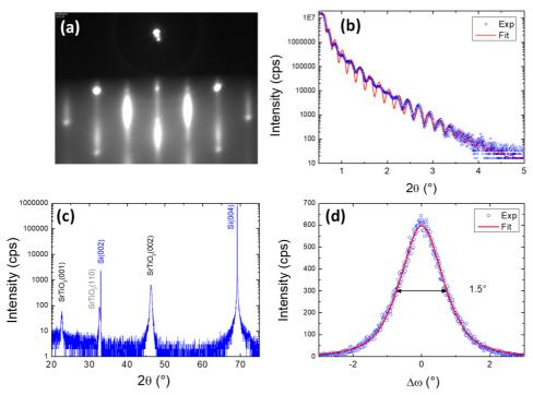
**Figure 1**: Structural characterization of the STO/Si substrate. (a) RHEED pattern recorded along the <100><sub>STO</sub> direction at the end of the growth, (b) XRR, (c) XRD  $\theta$ /2 $\theta$  scan, and (d) XRD  $\omega$ -scan around the (002) reflection of STO.
