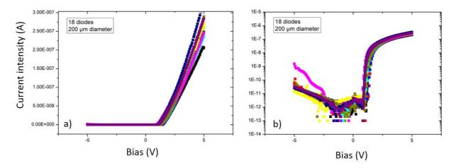
**Figure 14**: I-V characteristics of 18 diodes of 200 μm diameter at RT and under vacuum a) in linear scale; b) in logarithmic scale
