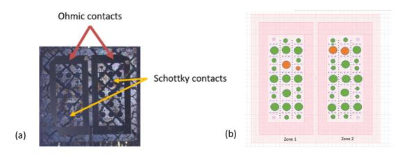
Figure 13 a) Optical image of the final device. Note that the cracks are located on the backside of the diamond crystal and seen by transparency (see details in the text); b) Mapping of the devices that present a diode behavior with rectification (in green) or (in orange) no rectification
