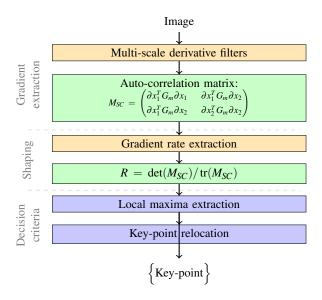
Figure 2. Steps to obtain full-vector-key-point detector.
