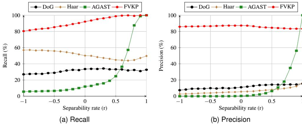
Figure 7. Complexity impact on the precision and recall.
