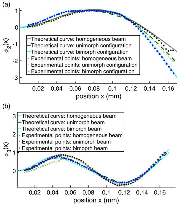
**Figure 7.** Comparison between the theoretically (lines) and experimentally (points) obtained second (top) and third (bottom) mode shapes for: the homogeneous beam (continuous line with cross points) without piezoelectric materials, the unimorph configuration (dashed line with x points), and the bimorph configuration (dotted line with star points).
