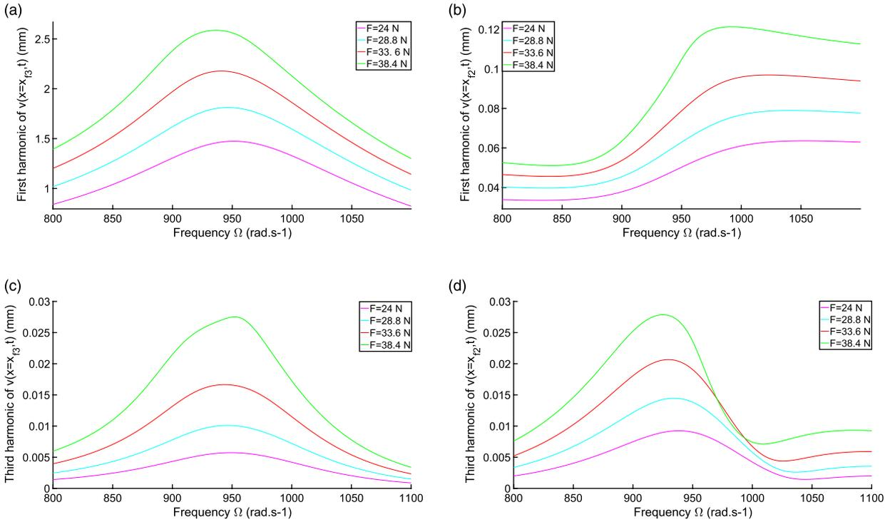
**Figure 4.** Theoretical results for the periodic forced response of the unimorph configuration in 1:3 internal resonance. Harmonics one and three of the displacements of the beam  $v(x = x_{f3}, t)$  (low frequency—mode 2—response, left column) and  $v(x = x_{f2}, t)$  (high frequency—mode 3—response, right column), as a function of the excitation frequency  $\Omega$ , for different amplitude of base acceleration (each color corresponds to a given base acceleration).
