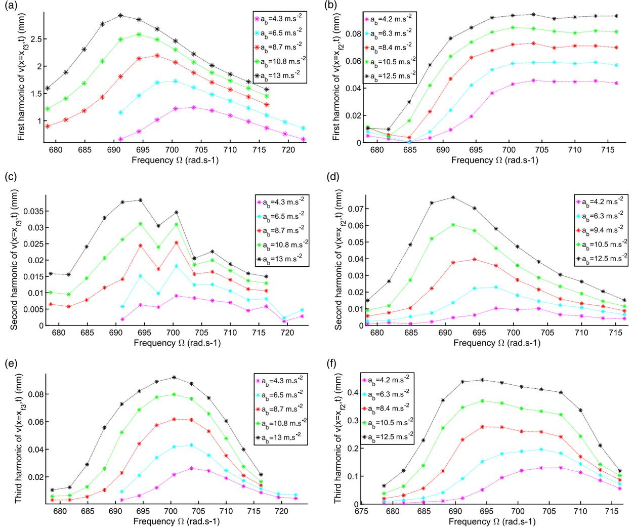
**Figure 9.** Experimental results for the periodic forced response of the bimorph configuration in 1:3 internal resonance. First three harmonics of the signals measured at  $x = x_{f3}$  (low frequency—mode 2—response, left column) and  $x = x_{f2}$  (high frequency—mode 3—response, right column) on the beam, as a function of the excitation frequency  $\Omega$ , for different amplitude of base acceleration (each color corresponds to a given base acceleration).
