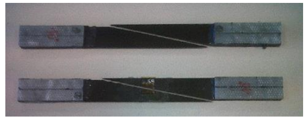
Figure 8 10^\circ Shear failure
