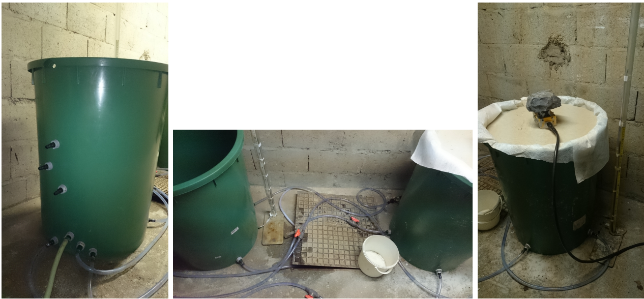
Figure 12. Pictures of the experiments. On the left is presented the tank filled with water, with its overflow connections. Middle picture shows the tubing linking both tanks. The picture on the right displays the sand tank with the GPR set at the top with a load on it.
